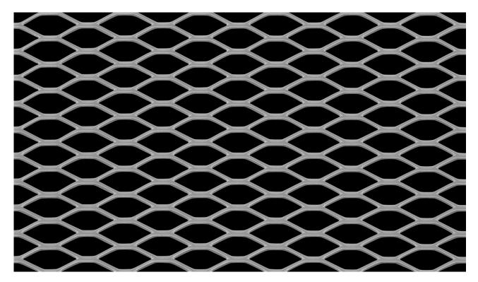
LW Pitch:28.58mmStrand Width:2.00mmSW Pitch:9.52mmThickness:1.20mmWeight:3.92 kg / m2Open Area:58%
